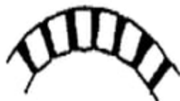
uncut bricks with wedge shaped mortar joints
