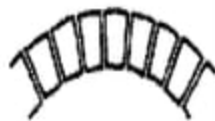
bricks cut to a wedge shape and mortar joints of uniform thickness
