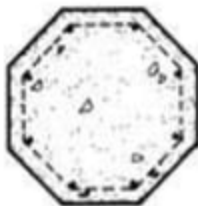
PRECAST CONCRETE PILE
