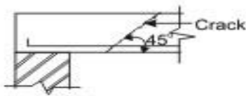
Figure 1.10 (a) Web shear progress along dotted lines
