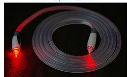
Fiber Optic Cable
