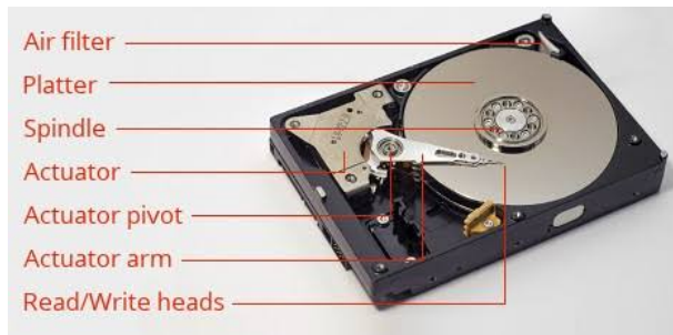
Fig.9: Components of hard disk drive
